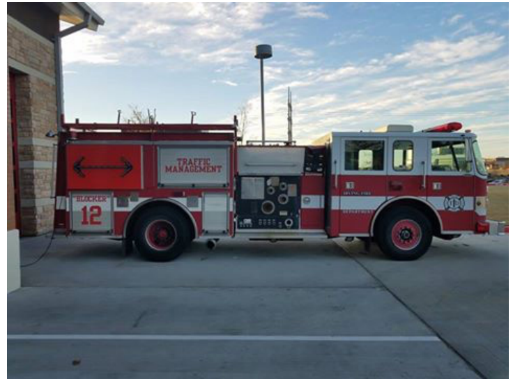
Figure 60 Refurbished Apparatus as a Block Vehicle from the City of Irving, TX
