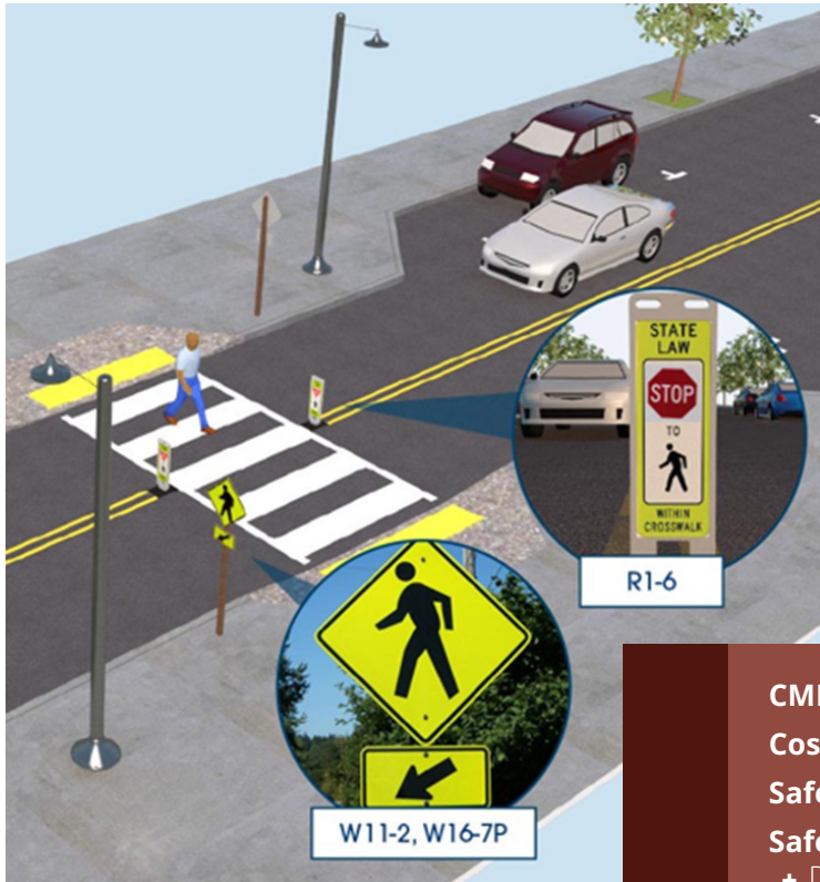
Figure 28 Crosswalk Visibility Enhancements
